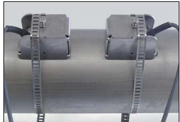
Flow transducers in transducer shoe, mounted with tension strap
