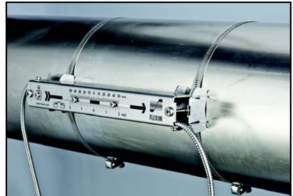
Measurement with transducers mounted with PermaRail
