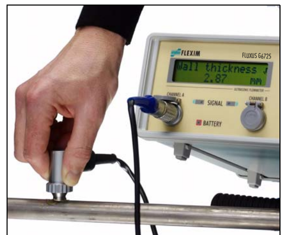
Wall thickness measurement (option)
